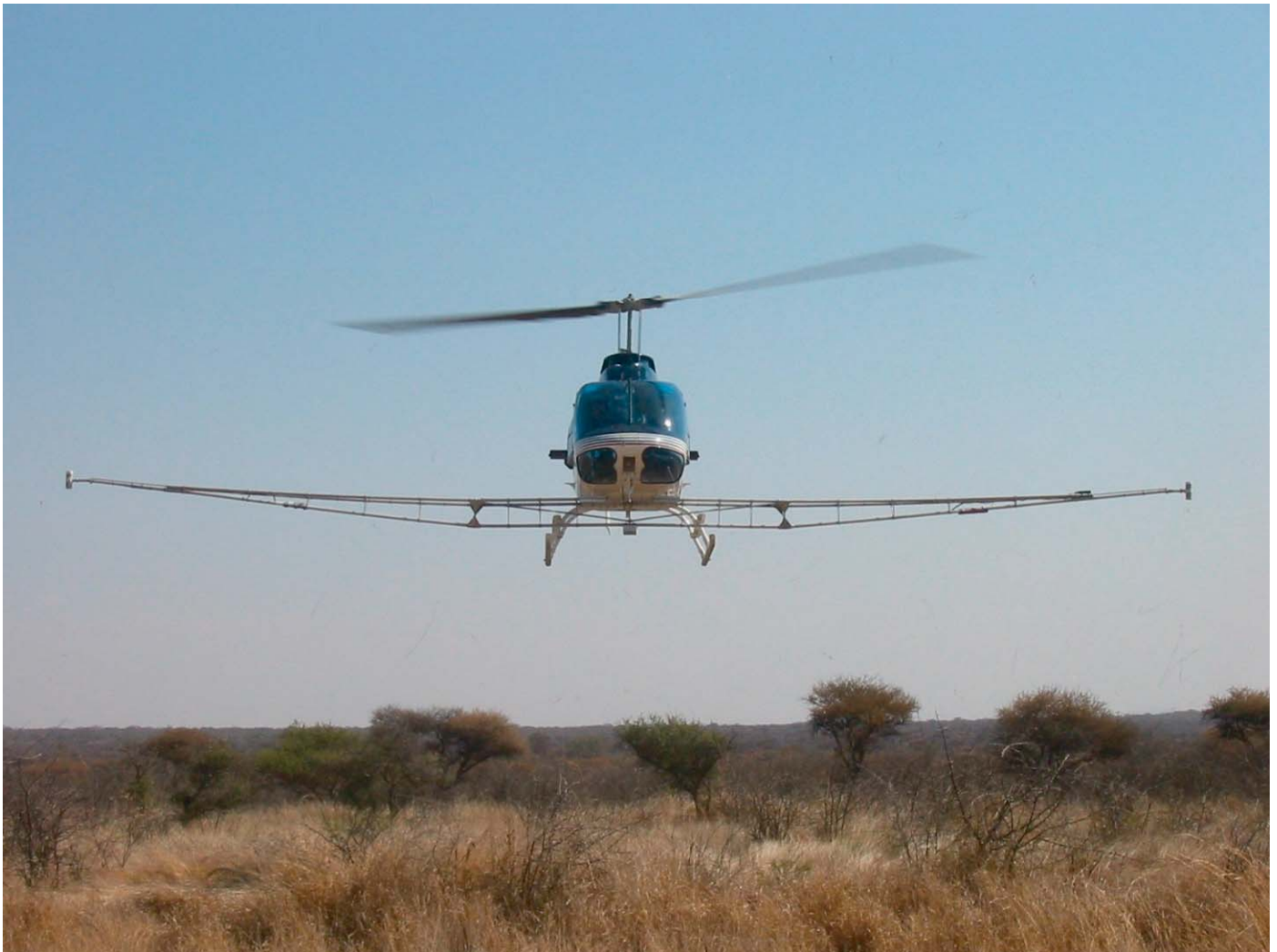
MIDAS™II Geomagnetic Mapping System Note the Horizontally Separated Sensors
